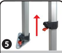
Lift two adjacent outer legs, push foot down to expose inner legs until you reach the snap lock holes. Repeat on all legs. To adjust height once snap locks are engaged, press down on red button to unlock. **NOTE:** Be sure all legs are set to the same snap lock holes.
