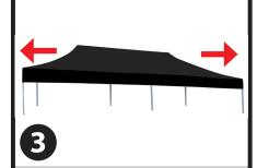
Expand frame out fully by having each person move to the middle leg of the 20' side. Grasp at bottom of the v. Lift up and step backwards at the same time until tent is fully opened.
