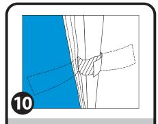
Attach the fastener around each leg on either side of the full wall.
