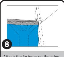
Attach the fastener on the edge of the full wall to the Fastener on the canopy.
