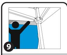
Continue attaching the fastener all the way to the end until the full wall is totally adhered to the canopy.
