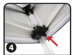
Engage the auto slider at each corner by pushing up with one hand while holding down top of leg with the other hand. Snap button will engage in groove. Repeat on all other legs. Attach the fastener in the corners of the graphic.
