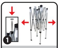
Insert truss bar into slot at center of frame. Place tent frame in center of final place. Pull frame outward (2 people recommended) from opposite sides while grasping legs. Lift off the ground and step backwards, stopping when 1/4 expanded.
