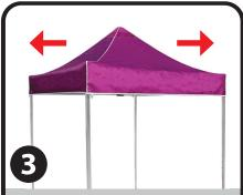
Expand the frame out fully by having each person stand on opposite sides, grasping the outer legs, lift up and step backwards at the same time until tent is fully opened.
