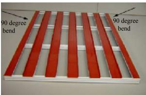
8. This image shows all the red stripes installed on the frame. All stripes should be under the clips and have red screws attached to the outter rafters at both ends. Before proceeding any farther check that the frame is square. By pushing on opposite cornors of the frame the frame can be squared.
