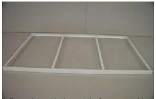
1. Frame Assembly: Lay out the frame assembly as shown, however place the square rafter holes facing down (not as shown-see next step) The two outside rafters should have the open channel facing in and the outter edge should be even with the ends of the U channel. The U channels have holes where the rafters should be positioned.
