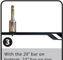
bottom, 23" bar on top, and spacer in between, marry the two bars together with the post.
