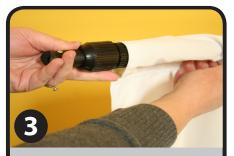
Before attaching other side of horizontal pole to the vertical pole, thread pole sleeve around horizontal pole. Then attach top horizontal pole to vertical pole like previous. If contour is not aligned with pole, turn telescoping joint clockwise to loosen and align.
