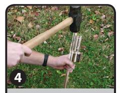
Hammer taller portion of the ground spike fully into the ground. Then insert pole with banner onto peg. For best vertical presentation, check with a level front-to-back and side-to-side.
