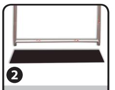
Using allen wrench, secure frame to steel base by tightening the aluminum studs.
