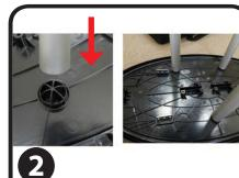
Insert the three poles into the base, then attach the top part.
