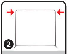
Then lay the frame down and insert the center rods.
