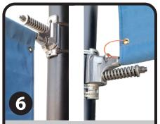
Secure banner to Bracket by threading a Zip Tie through both banner grommet and Spring Clip as shown above. Lock the Zip Tie by inserting it's tip into it's head until it clicks at least twice.
