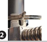
Attach the upper Mounting Strap loosely to the post at the desired height. Slip the Top Bracket behind the Strap. The spring will be above the Rod hole. Place the Strap onto the Bracket's flange and into the channel.
