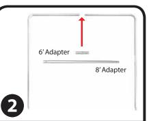
Select the correct Adapter for the table top size. 6' tables will use the short (5") Adapter. 8' tables will need the long (28"). Position the Adapter between the side supports and join the two supports together, connect with snap buttons.
