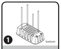
Remove straps, open trunk and remove parts. Turn trunk bottom upside down. Push legs into holes located on the trunk bottom.
