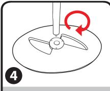
Align assembled parts over the base and screw clockwise.
