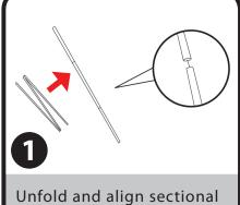
Unfold and align sectional tube frame.
