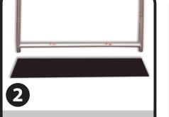
Using allen wrench, secure frame to steel base by tightening the aluminum studs.
