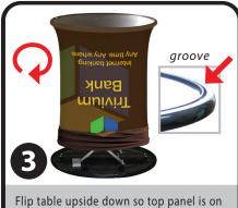
the floor. Holding the bottom hem of the graphic, find the back seam and feel for the rigid cord inside the hem. Line up the back seam with the middle of one long side of the bottom panel and push the cord into the groove on the bottom panel.
