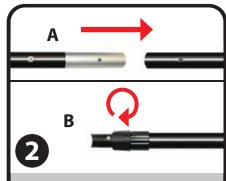
**A:** Pick up one short pole w/flat end and one short pole w/silver end and snap together. Repeat with remaining short poles.
