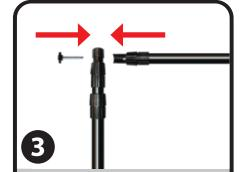
Align contoured end of pole assembled in step #2 to the hole in the top of one vertical pole. Insert winged bolt through the hole and into the threaded hole of the contoured end. Screw winged bolt until tight.
