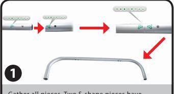
Gather all pieces. Two S-shape pieces have strings that connect four segments. Align pieces & push together until metal tabs lock in place. Assemble pieces by lining up matching stickers & pushing hardware pieces together until metal tabs lock in place.
