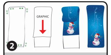
Place graphic above hardware & slide over the Wave shape, pulling left & right sides evenly downward. Once graphic is two-thirds down the Wave shape, pull the top of the graphic onto the Wave shape. Then pull from the bottom of the graphic to the floor. Note: You may find this step easier to complete with two people.
