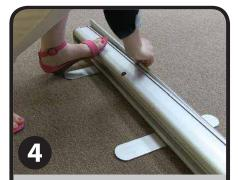
Stand at the back of the Base and begin to gently pull the banner upwards. Clip the hook at the top of the assembled Sectional or Telescoping Pole to edge at the top of the banner.
