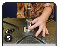
Still holding the screw in place on the underside of the tank, place the peg on the screw on the top of the tank. Holding the base of the peg, twist the peg clockwise until it is secured.
