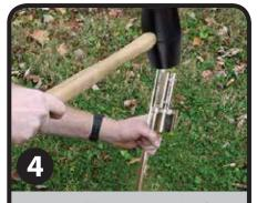
Hammer taller portion only of the ground spike fully into the ground. Then insert pole with banner onto peg. For best vertical presentation, check with a level front-to-back and side-to-side.
