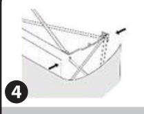
Line up fastener on banner to hardware and affix banner to hardware. Banner should be taut when completely affixed to hardware. IMPORTANT: When taking kit down make sure to verify that ALL hooks have been disconnected from each other.
