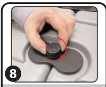
Tighten the Base Connector bolt on to nut to fasten both Quadrants. Repeat steps 5 to 8 for the remaining Connectors.
