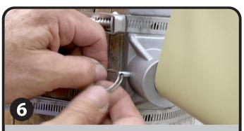
Thread the retainer rings through the hole in the end of each of the clevis pins.
