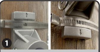
Each bracket is marked with a directional arrow. The arrow should be pointing up for the top bracket and down for the bottom bracket.
