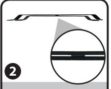
Place 23" bar on top, sandwiching the spacer between both bars. Align holes.
