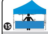
Align bar to be parallel with the ground and use snap locks to pull out exterior bars to reach clamp. Secure with thumbscrew and hex nut.
