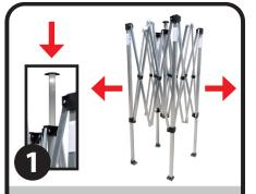
Insert truss bar into slot at center of frame. Place tent frame in center of final place. Remove strap and have two people stand on opposite sides. grasping the outer legs. Lift off of ground and step backwards, stopping when about 1/4 expanded.
