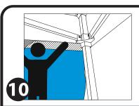
Continue attaching the fastener all the way to the end until the full wall is totally adhered to the canopy.
