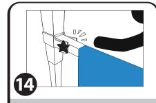
Place first clamp on leg. Insert half wall pole into clamp. Slide thumbscrew through clamp and pole into the hex nut. **Do not over tighten.** Attach second clamp on connecting leg.
