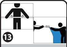
Connect two half wall poles until they snap together. Slide the assembled half wall pole through the pole sleeve of the half wall.
