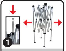
Insert truss bar into slot at center of frame. Place tent frame in center of final place. Remove strap and have two people stand on opposite sides, grasping the outer legs. Lift off of ground and step backwards, stopping when about 1/4 expanded.
