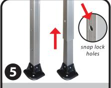
Lift two adjacent outer legs, push foot down to expose inner legs until you reach the snap locks. Repeat on all legs. Raise or level the tent using adjacent holes found near bottom of each outer leg. NOTE: Be sure all legs are set to the same snap lock holes.
