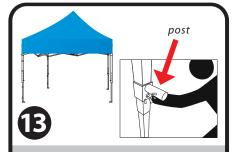
To attach half wall connectors to the tent leg, pull down on the inner leg of the tent leg to remove it from the tent frame. Slide half wall connector onto the tent leg, being sure the post of the connector points where the half wall will hang. Reinsert the inner leg. Repeat on second leg.
