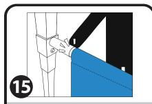
Attach both ends of the pole to the half wall connectors.
