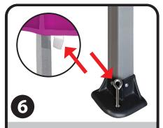
If added support is desired (on soft surfaces): Thread rope through a sewn-in tab of the canopy down to the ground stake below.
