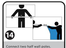
Slide the assembled half wall pole through the pole sleeve of the half wall.
