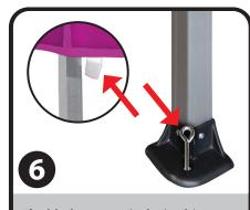
If added support is desired (on soft surfaces): Thread rope through a sewn-in tab of the canopy down to the ground stake below.
