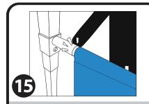
Attach both ends of the pole to the half wall connectors.
