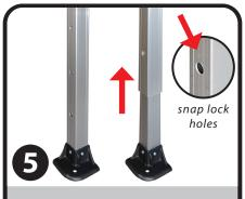
Lift two adjacent outer legs, push foot down to expose inner legs until you reach the snap locks. Repeat on all legs. Raise or level the tent using adjacent holes found near bottom of each outer leg. **NOTE:** Be sure all legs are set to the same snap lock holes.
