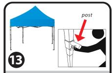
To attach half wall connectors to the tent leg, pull down on the inner leg of the tent leg to remove it from the tent frame. Slide half wall connector onto the tent leg, being sure the post of the connector points where the half wall will hang. Reinsert the inner leg. Repeat on second leg.
