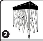
Place tent graphic over frame. DO NOT attach the fastener in the corners.
