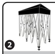
Place tent graphic over frame. DO NOT attach the fastener in the corners.
