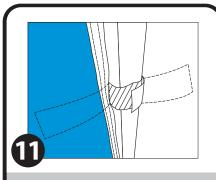
Attach the fastener around each leg on either side of the full wall.
