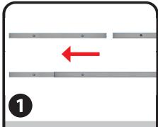
Line up short pole w/snap lock and one long pole as shown above. Depress snap lock and slide short pole inside long pole until snap lock is engaged. Repeat with remaining snap lock and second long pole.
