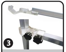
Remove hand screws from one clamp. Insert medium pole w/peg into half of clamp lining up holes. Place clamp w/ pole onto tent leg just below canopy. Line up second half of clamp, insert hand screws and tighten. Repeat with second clamp on next tent leg.
