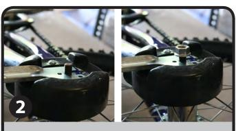
Mount the base of the flag on the rear axle of the bike.
