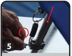
Attach one ring of the Spring Assembly to the Hook from step #4. Attach remaining ring over the Tension Knob. **Gently**, slide Tension Knob downwards until desired tension is achieved. Tighten Knob.
