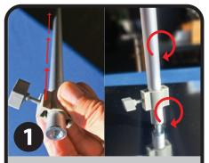
Slide Tension Knob onto the bottom segment of the Center Post. Line up Center Post with hole in top of base. Attach Base Bolt through the Base from the bottom and into the Center Post. Tighten Bolt.
