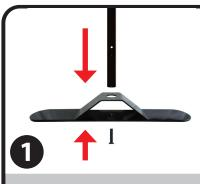
Position one foot next to one long pole. Insert pole into the hole located on the top of the foot. Thread one screw (found in bag with small parts <u>OR</u> pre-threaded in long pole) through the hole in the bottom of the foot and into the pole. Tighten with allen wrench.
