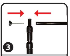
Align contoured end of pole assembled in step #2 to the hole in the top of one vertical pole. Insert winged bolt through the hole and into the threaded hole of the contoured end. Screw winged bolt until tight.
