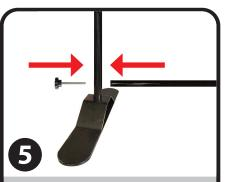
Pick up second pole assembled in step #2 and align contoured end to the hole in the bottom of one vertical pole.
