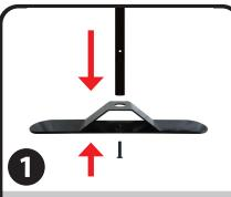
Position one foot next to one long pole. Insert pole into the hole located on the top of the foot. Thread one screw (found in bag with small parts <u>OR</u> pre-threaded in long pole) through the hole in the bottom of the foot and into the pole. Tighten with allen wrench.
