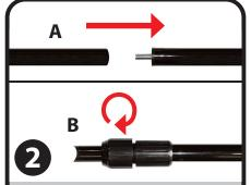
**A:** Pick up one short pole w/flat end and one short pole w/screw end and screw together. Repeat with remaining short poles.
