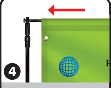
Before attaching the top pole to the second vertical pole, slide the top pole sleeve of the graphic onto the pole.
