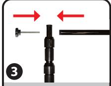
Align contoured end of pole assembled in step #2 to the hole in the top of one vertical pole. Insert winged bolt through the hole and into the threaded hole of the contoured end. Screw winged bolt until tight.
