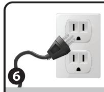
Insert plug from Illuminator InstaStand into electric socket. Be careful to place the cord where no one will trip over it.
