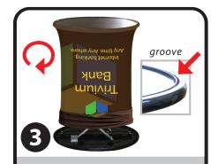
Flip table upside down so top panel is on the floor. Holding the bottom hem of the graphic, find the back seam and feel for the rigid cord inside the hem. Line up the back seam with the middle of one long side of the bottom panel and push the cord into the groove on the bottom panel.
