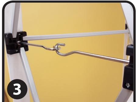
Interlock central, front-side and back-side hooks followed by hooks on top then bottom. This may require assistance. For greater leverage, lay the frame flat on the floor to interlock hooks.
