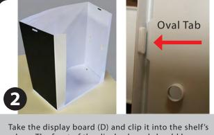
Take the display board (D) and clip it into the shelf's edges. The front of the display board should be aligned with the arc of the shelf's base. There are oval tabs on the base shelf that will align with the oval shaped holes on the display board. Be sure to fold the white flaps of the board so that they are tucked into the ridges along the backside of the base shelf.
